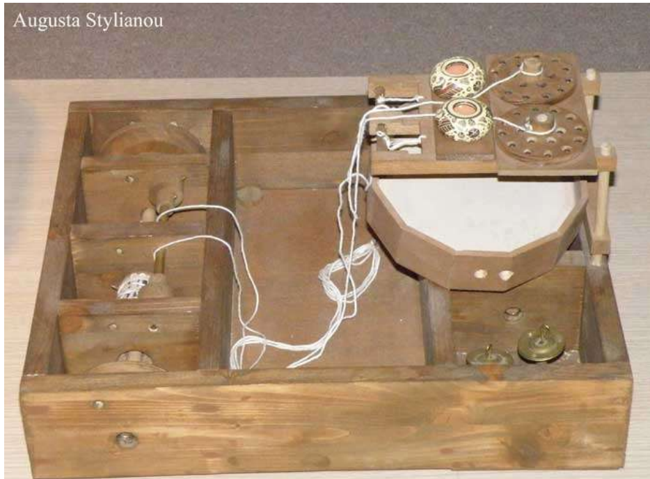
Figure 24. Part of the mechanism for Heron's Automatic Theater illustrating the programmed controls for drumming and cymbals (metal balls held in perforated wheels on the upper right of the mechanism are dropped one-by-one onto the drumhead as the attached cord is wound onto a shaft, where they then roll through one of the hole in the drum mechanism and fall onto the cymbals). The lengths of the strings and the way they are wound on pegged shafts controls the sequence of events 120 . The mechanics of the operation are shown and explained more clearly on a detailed video of the complete mechanism. (from Hellenica's Ancient Greece/Science and Technology ).
