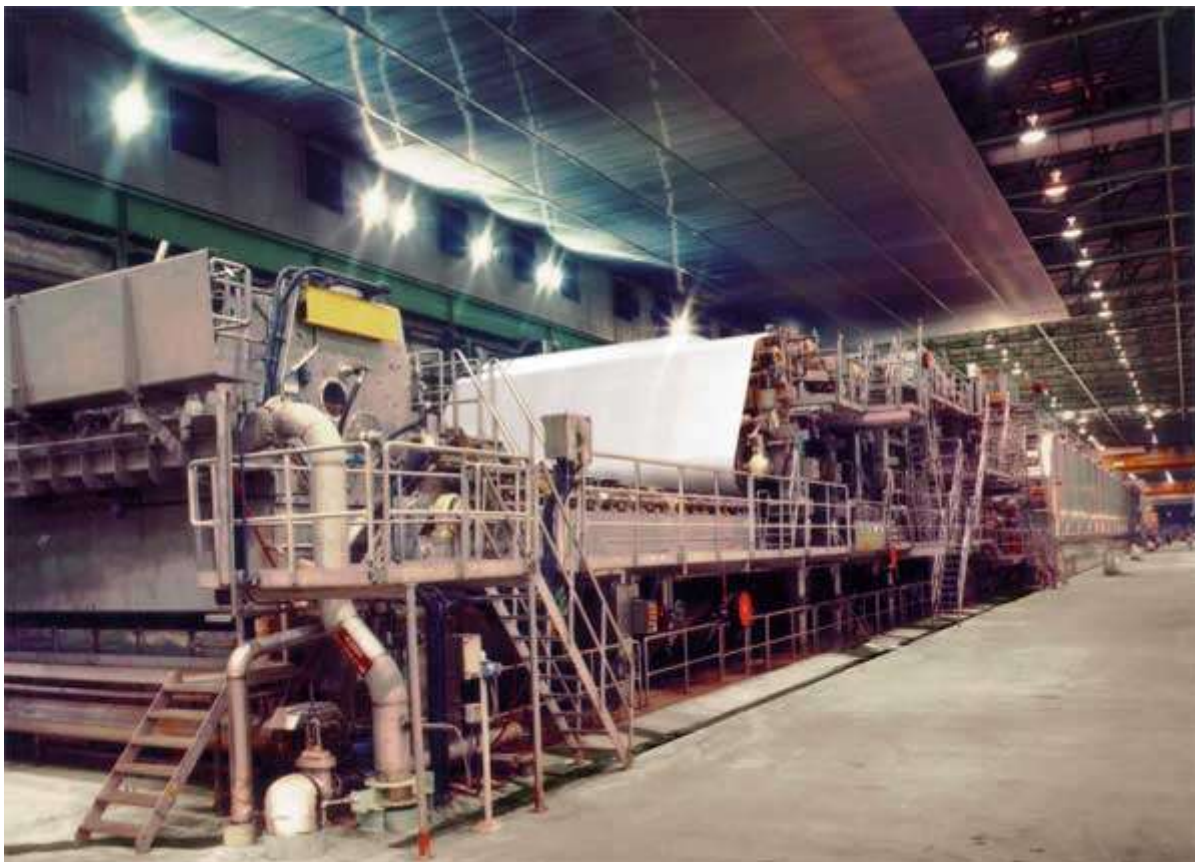
Figure 17. The "wet end" of a modern Fourdrinier paper making machine where a slurry is spread on a fine wire screen to begin draining the water and consolidating the fibers. The far end of the dryer and the take-up reel is lost in the distance.
