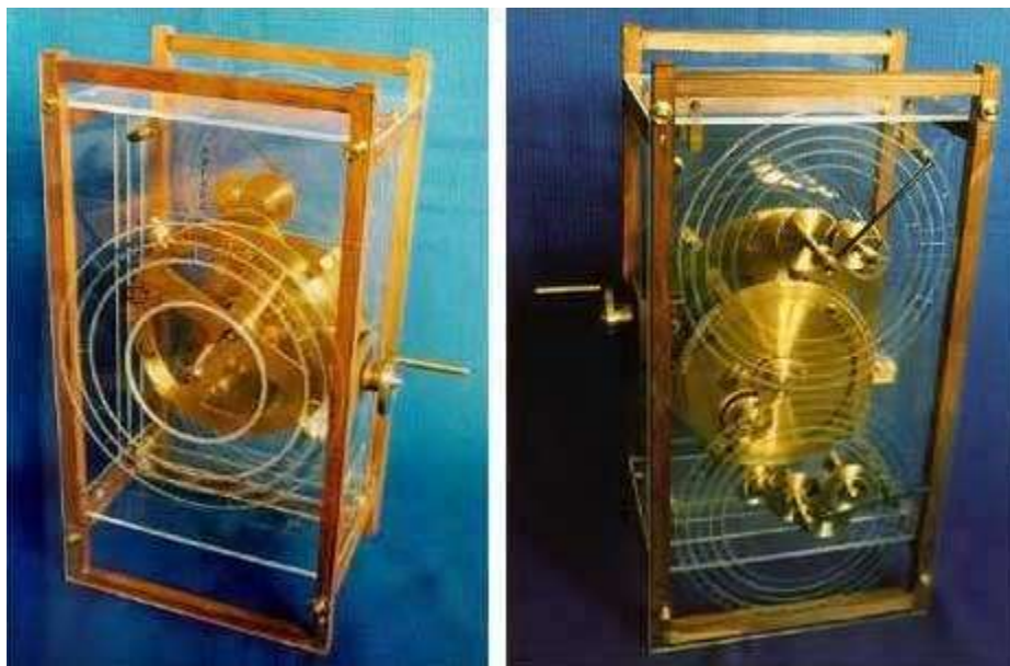
Figure 23. Reconstruction of the Antikythera Mechanism. A full scale version by John Gleave, Orrery Maker , based on the Price ( 1959 ) reconstruction. Height 12.25 inches. Left: The front dial - showing the annual progress of the sun & moon through the zodiac, against the Egyptian calendar, rendered in Greek on the outer annulus (In the latest reconstructions, the front dial includes at least 10 more gears and five more pointers for the planets known to the Greeks - Freeth et al. 2006 , 2008 , Freeth & Jones 2012 ). Right: The back dials. The upper back dial displays a four year period and has five concentric inscribed rings, most probably each with 47 divisions giving the Metonic Cycle of 235 synodic months, which equals 19 solar years. The lower back dial gives the cycle of a single synodic month, and the subsidiary dial the Lunar year of 12 synodic months (Pictures from Grand Illusions).
