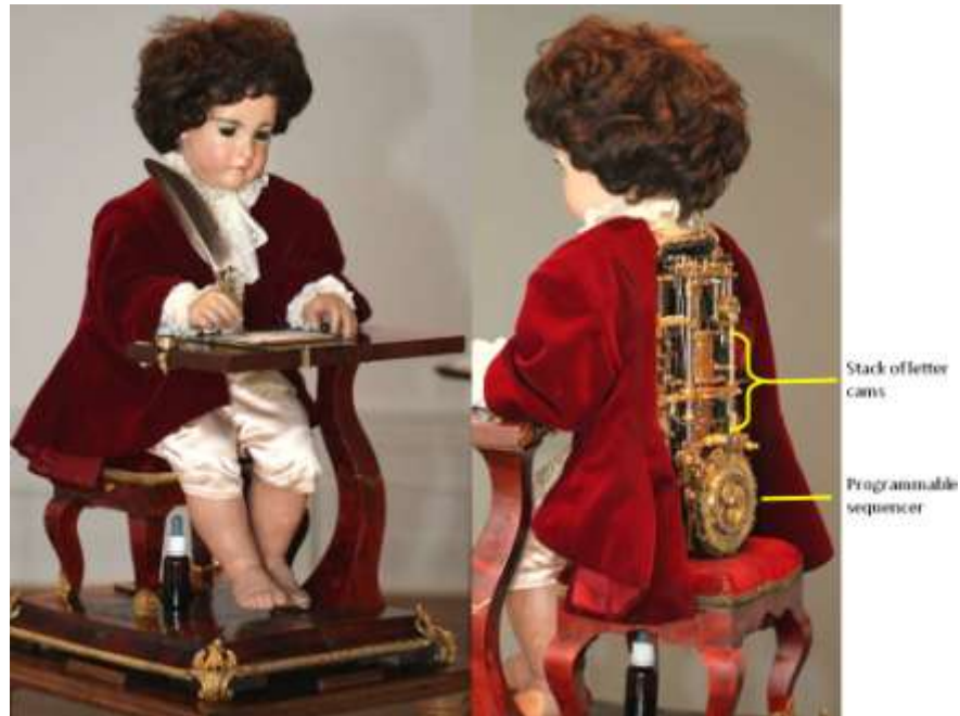
Figure 26. The Writer automaton, constructed from around 6000 components between 1768 and 1774 by Pierre Jaquet-Droz, his son Henri-Louis, and Jean-Frédéric Leschot in Switzerland (From Miklós 2013 ).
