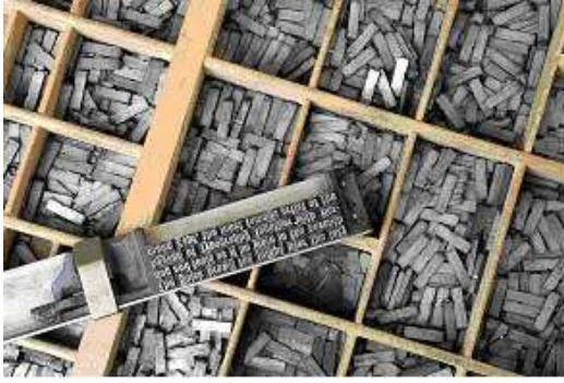
Figure 18. Hand setting type of a particular type font from the type case. The case has two major divisions (or there may be two separate cases used at the same time), where the “upper case” contains capital letters, and the “lower case” (closer to the typesetter) contains the small letters. The arrangement of boxes in the cases is standardized, with the size of the box for each letter based on how commonly used it is.
