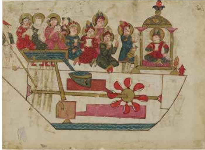
Figure 25. Ibn al-Razzas Al-Jazari's autonomous musical toy (Smithsonian via Wikipedia). A video by MTE Studios based on Al-Jazari's written explanation demonstrates how it worked 121 .
