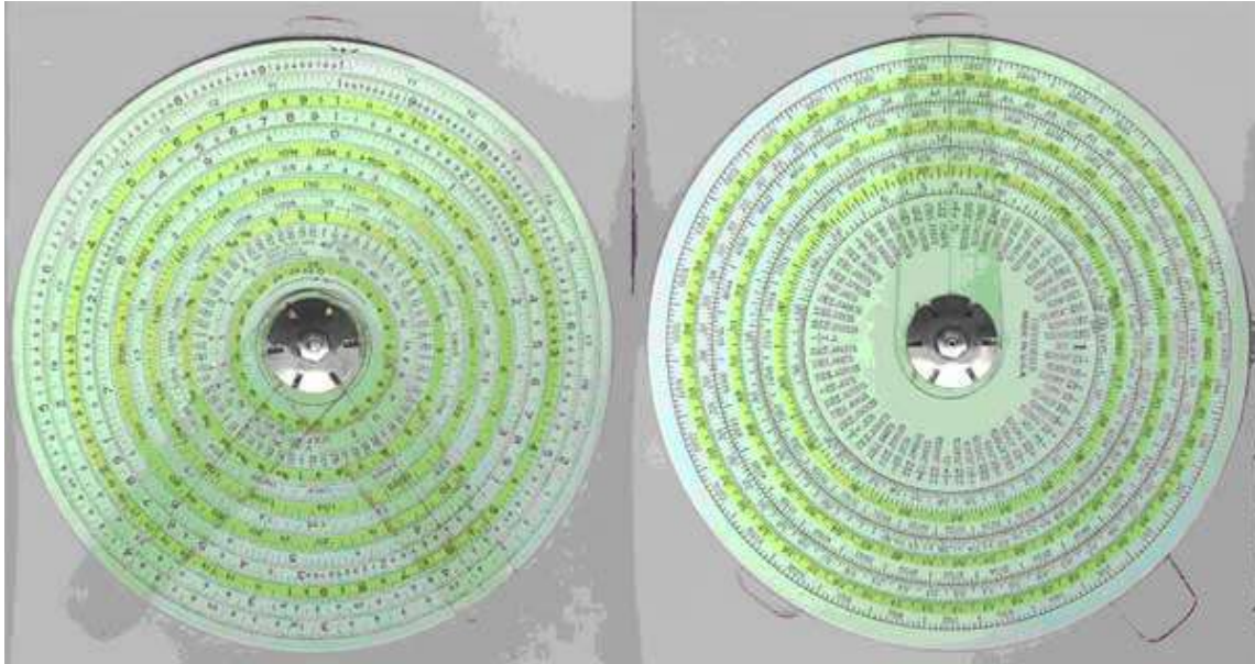
Figure 29. Dietzgen 1797B (Gilson Binary) 21.1cm dia. Made in USA by Gilson for Dietzgen. Front Scales: C, CI, A, K, Log, LL1, LL2, LL3, LL4, Binary, Fraction, Drill thread, Millimeter; Back Scales: Degrees, S, T, Degrees, S, T, Degrees, S, T, Fractions (Click picture for enlarged view - International Slide Rule Museum )
