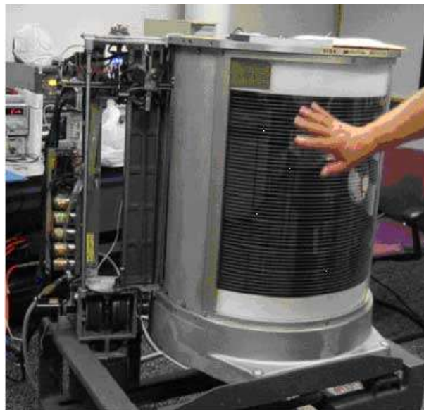
Figure 36. IBM's 350 magnetic storage unit that was the heart of the 305 RAMAC (Random Access Memory Accounting) system ( Wikimedia Commons ). 50 disks with 100 recording surfaces provided 3.75 MB storage at a lease cost of 3,200/month. See IBM's advert showing the system in action.
