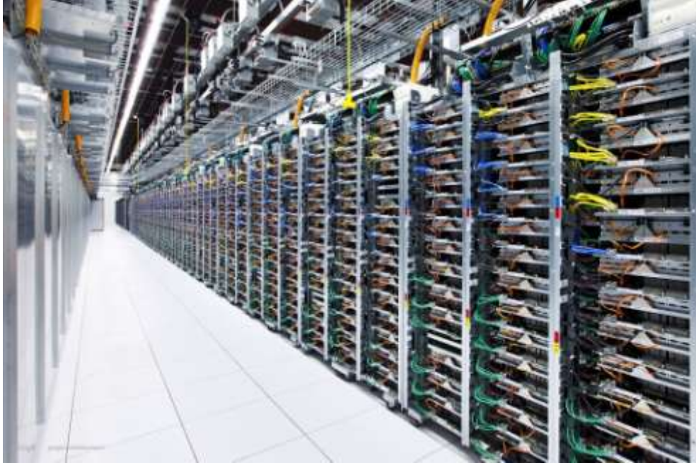
Figure 45. A small part of one of Google's data centers 224 . Each rack holds 15 server boards ( Google Data Centers , photo gallery ).
