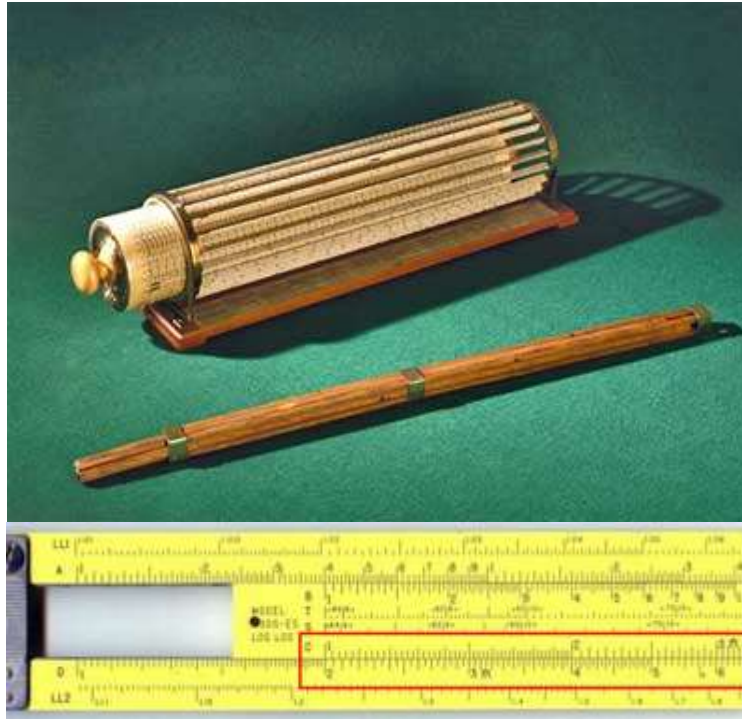
Figure 28. Slide rules. Top - Thacher's slide rule, an important American contribution to slide rules, capable of accurate reading to four decimal places (Science Museum/Science & Society Picture Library). Middle – the first slide rule design after Oughtred, made by Robert Bissaker, 1654. Bottom - A slide rule positioned so as to multiply by 2. Each number on the D (bottom) scale is double the number above it on the C (middle) scale (Wikimedia Commons Benjamin Crowell).
